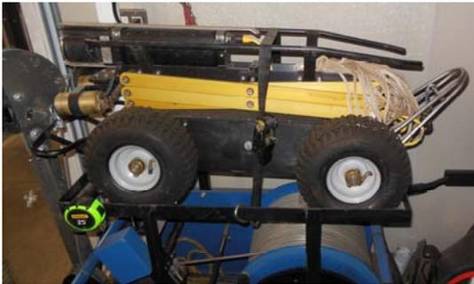
Large sewer camera with capability of extending height of camera to minimize potential for submersion.
