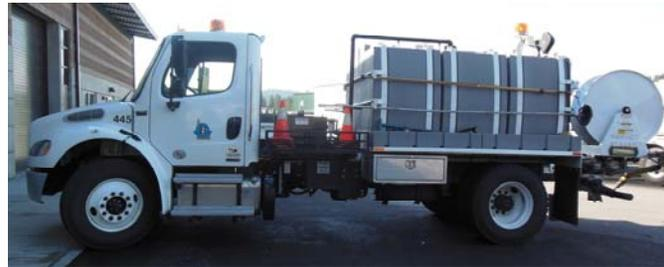
“Little Jet” Jet Truck– uses hydraulic water pressure up to 2000 psi to clean City sewer lines.
