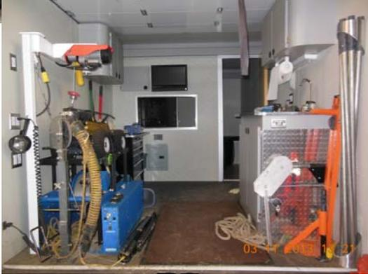
Inside the "TV Van," is a mobile office with equipment that has the capability of taking video of sewer line between 6"-36" in diameter. As video is recorded, it can then be transferred to disc for further viewing or archival.
