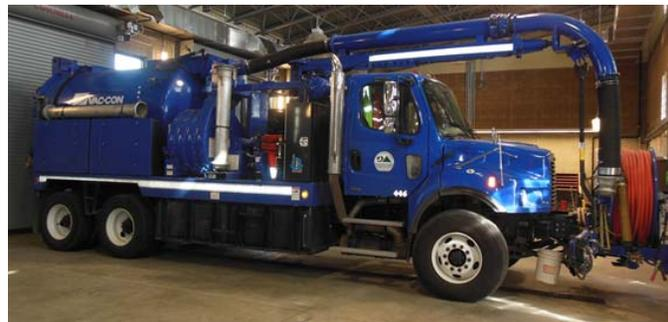
“Big Blue” Jet Truck– like the “Little Jet, Big Blue” uses hydraulic water pressure (2000 psi) to clean City Sewer lines. The difference between the two is, “Big Blue” also has the ability to vacuum debris out of the sewer line.
