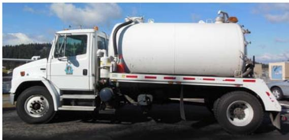
“Tank Truck” cleans the City sewer line by using 2000 gallons of water to flush the line.
