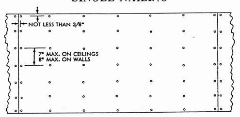
"SINGLE NAILING" SYSTEM PROCEDURE: The wallboard shall be held in firm contact with the nailing member while the nails are being driven. Nailing preferably should proceed from the central portion of each piece of wallboard towards ends and edges. Nails shall not be staggered on adjoining edges or ends. Perimeter nailing at the top and bottom is not required.
